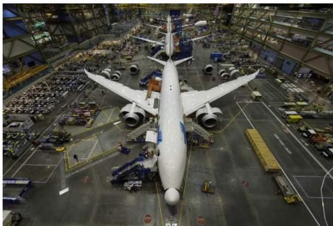
The 787 Dreamliner, with its 50% carbon fiber reinforced plastic airframe, being manufactured at Boeing's factory in Everett, Washington. (Picture © Boeing.)
