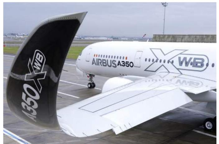
Around 50% of the new Airbus A350 XWB is constructed of carbon fiber composite, including its aerodynamic wings. (Picture © Airbus S.A.S. 2014 – photo by master films/A. Doumenjou.)
